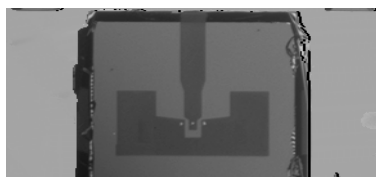
Figure 3 Photograph of probe window with GCPW to microstrip transition for on-wafer probing.
